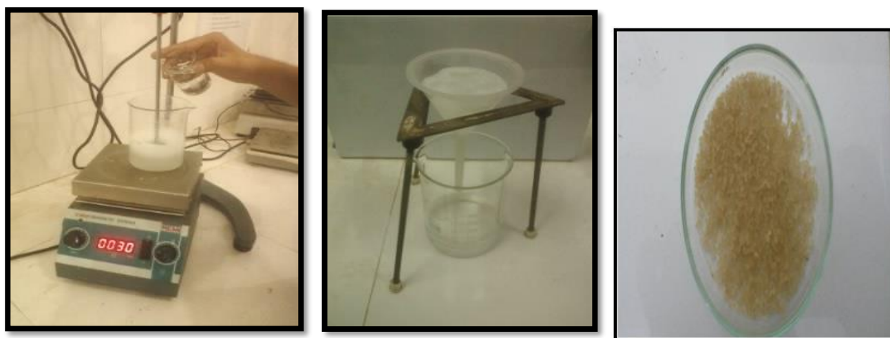
Figure 13: Preparation of mucoadhesive microspheres
